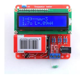
For resistors below  $2100\Omega$  also the measurement of inductance will be done. The range will be from about 0.01mH to more than 20H, but the accuracy is not good. The measurement result is only shown with a single component connected.
